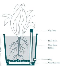
Always use the planter in conjunction with the liner and remove the plug at the base of the liner and the base of the planter if the planters are going to receive rainfall.
